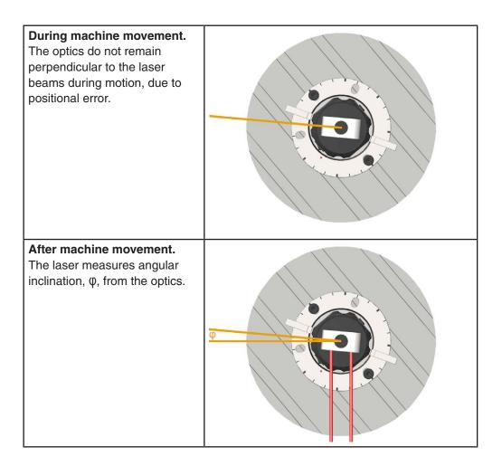
3. Monitoring machine movement to distinguish when the machine is stationary and capable of recording a position. Due to machine vibration and other environmental factors the setup will never remain perfectly stationary. The laser monitors when the machine has reached its target position by recording when the system is within angle  $\alpha$ . It also recognises when the machine is 'stationary' by monitoring the laser readings until they have become stable.
