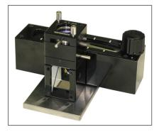
The latest version of the straightness base (shown opposite) is required to perform measurements using the fixed turning mirror and beam steerer.
