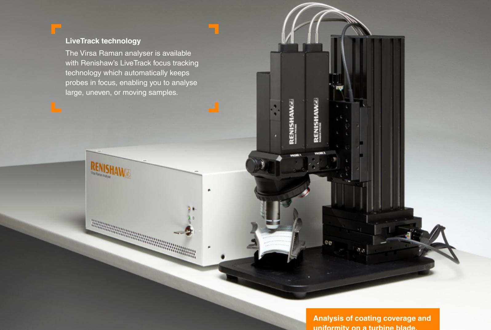
Analysis of coating coverage and uniformity on a turbine blade.
