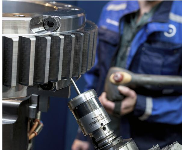
Renishaw RMP60 probe confirming finished gear dimensions after deburring
