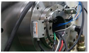
Figure 3. DDR rotary table application with RESOLUTE encoder in-situ (ITRI, Taiwan).
