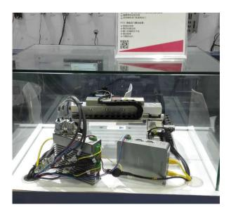
Figure 1: exhibit of the ACS test stage with the RESOLUTE encoder onboard
