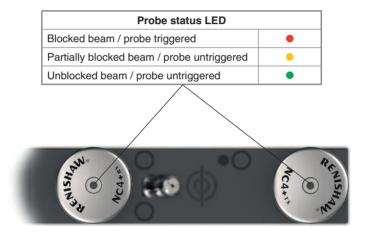
For more information on these LED sequences and modes of operation, see the *NC4 non-contact tool setting system* installation and maintenance guide (Renishaw part no. H-6270-8501).
