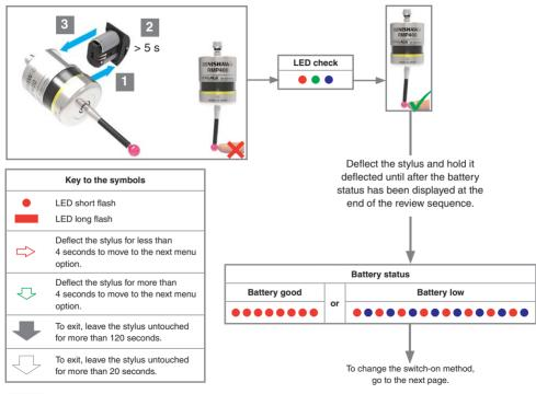
**CAUTION:** Do not remove the batteries whilst in configuration mode. To exit, leave the stylus untouched for more than 20 seconds.
